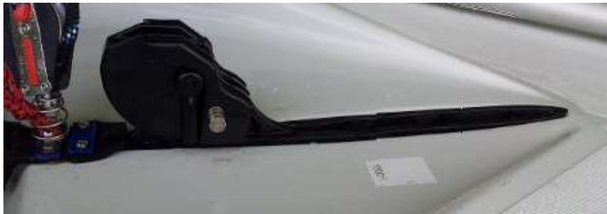
Fig 14 Gear block with retaining pin inserted through the centrecase insert. GF007
