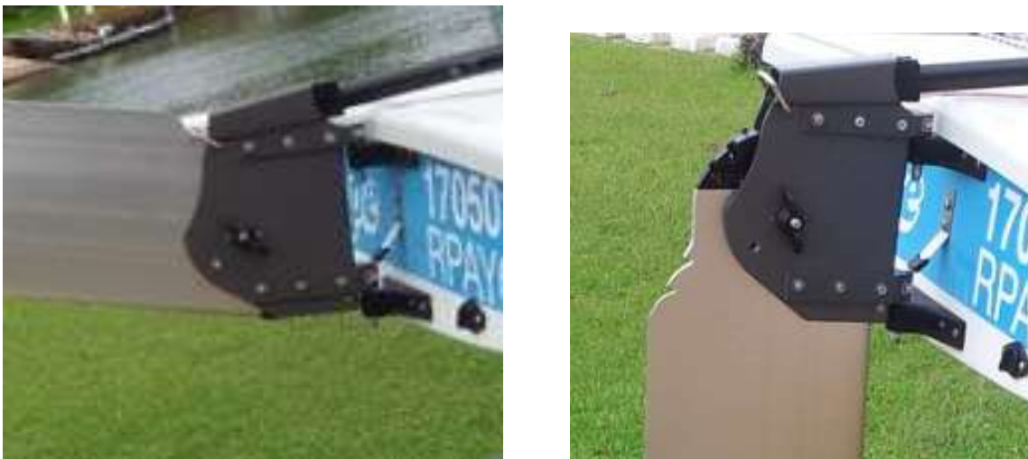
Fig 31 Showing the rudder blade in the retracted position and fully deployed
