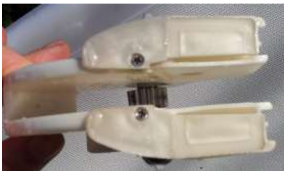
Fig 15 Gear block with packers attached with screw
