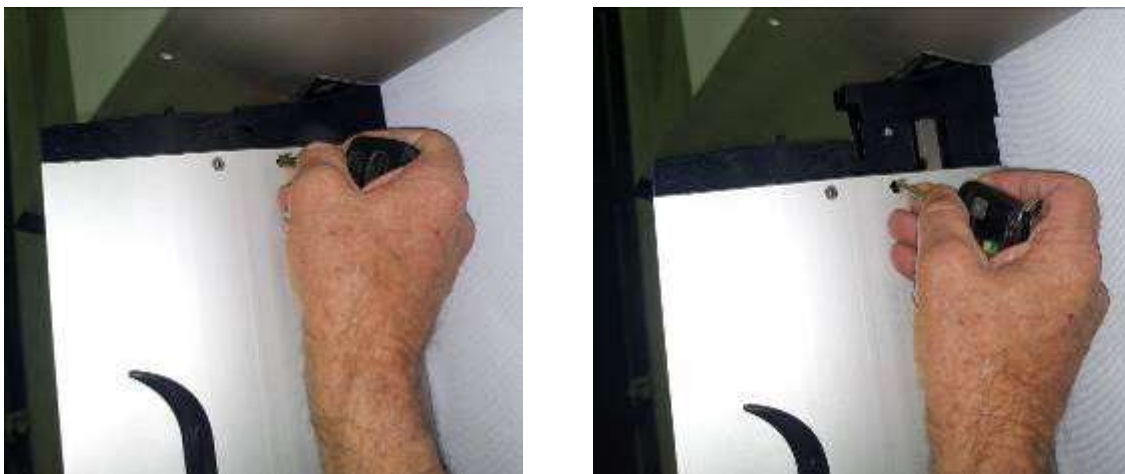
Fig 18 Depress the spring clip and pull the foils apart.
