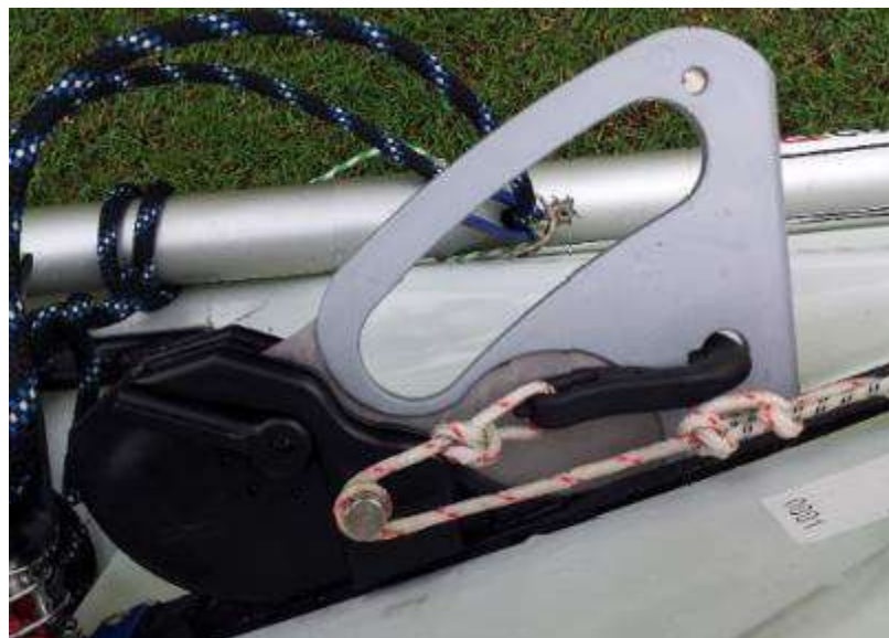
Fig 22 Once engaged in the gear block, rotate the large retaining clip 180 degrees and wrap the cord around the pin with one complete turn as shown.
