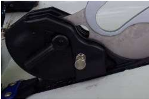
Fig 23 &24 Rotate the gear handle part way, prior to engaging the handle.
