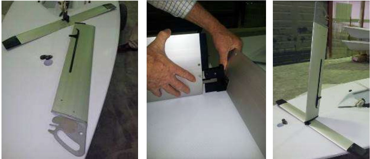
Fig 17 Assembly of Centreboard foil GF001 and lifting foil GF002
