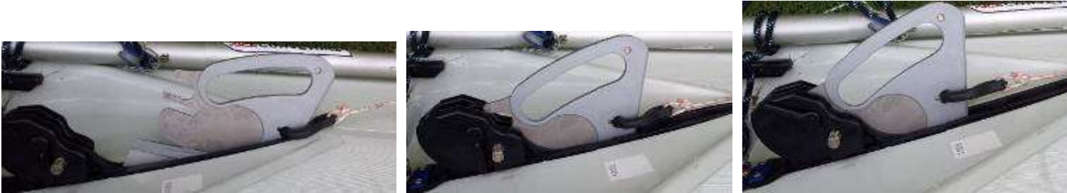
Fig 21 Pull board down and aft to engage in gearblock. Pull the board down until the clip sits on the deck, then pull the board backwards to engage the gear block.
