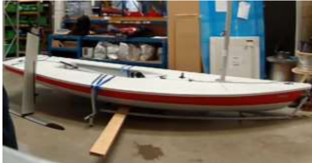
Fig 13 Method to support the centrecase insert from below when fitting the gear block.
