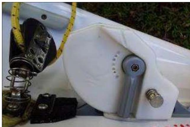
Gearblock with toggle pin attaching to the insert.
