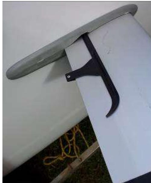
Wand mechanism retracts within the centre case for easy launching and retrieval
