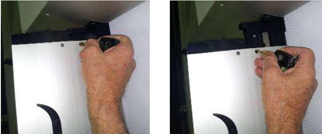
Simply depress the spring clip and pull the foils apart.
